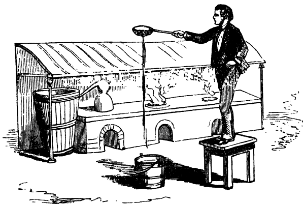
Fig. 265. Process of granulating Zinc by pouring it from a height into a pail of cold water.
